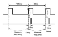
If the period of the external input is less than the setting of the delay time, the delay time is ignored and the ST-329 flashes as if the delayed time equals 0.
