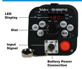
Store and retrieve 5 flash setting values LOAD Change Operation from INTERNAL to EXTERNAL SIG flash control Select between Flash Mode or Flash Duration MODE and phase shift settings Multiply or divide Flash Rate Setting by X2 or +2 Select between degrees or ms in phase shift mode, **UNIT** select between degrees and  $\mu$ s in flash duration mode
