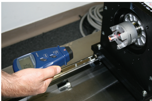
PT-110 recording rotational speed of machinery.
