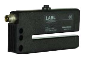
The LABL sensor combines small spot size and fast response to achieve high-speed label detection. The LABL is capable of detecting a wide variety of adhesive labels on various backings. The Learn key provides Standard, Thin and Custom Learn. Custom Learn (LABL-2) provides a separate measurement on the gap and on the label to allow for optimal detection of difficult labels.
