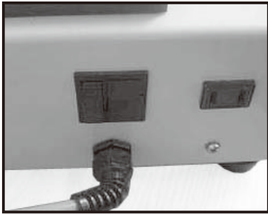
AC Power cord and AC plug for the Force gauge, located on the back of the rear of the test stand.
