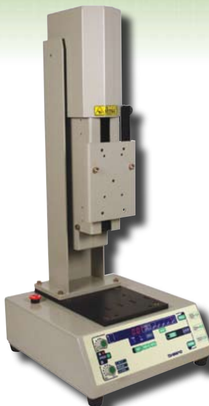
Series FGS-100PV Vertical Motorized Test Stand
