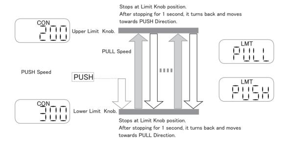
Change speed by UP, DOWN Key. SIg Mode and CON Mode Speed Setting are commonly used. During movement, speed variation is not possible. When no movement is occurring (at idle), the display shows movement Mode and the latest operated speed. When the movement starts, the respective memorized movement . Speed is displayed.
