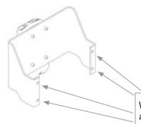
With the 4 Installation bolts, install the Force Gauge and Mounting Bracket to the Test Stand
