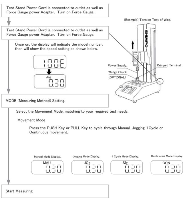
With the PUSH or PULL Key, Measurement can be started. For details refer to the Movement Mode Operation described later. Load Tests as follows can be performed.
