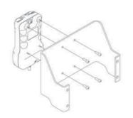
Using the Allen wrench spanner provided in the accessories, remove the installation bolts connecting the Test Stand and the Force Gauge Mounting Bracket
