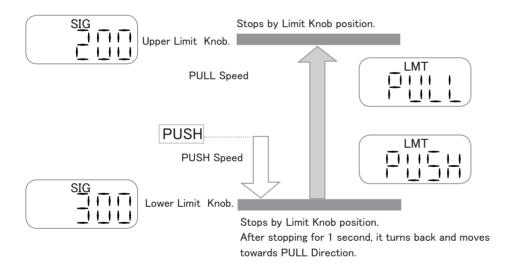
Change speed by UP, DOWN Key. SIG Mode and CON Mode Speed Setting are commonly used. During movement, Speed variation is not possible. When no movement is occurring (at idle), the display shows movement Mode and the latest operated speed. When the movement starts, the respective memorized movement speed is displayed.
