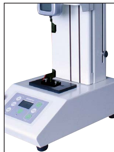
Stand with Optional Grip Performing Tension Test
